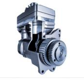
The **compressor with coupling** automatically uncouples from the engine when the system is adequately supplied with air, thus lowering a truck's CO<sub>2</sub> emissions by about 2.5 metric tons per year.
