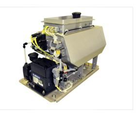
New **sanding systems** reduce to a minimum the fine dust produced when braking rail vehicles and also come with modern diagnostic options.
