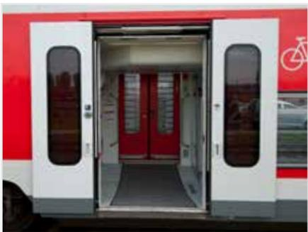
The **IFE Generation 4 Entrance System** is 20% lighter and uses 25% less energy than its predecessor. New materials for the door leaves have improved levels of noise and heat insulation.
