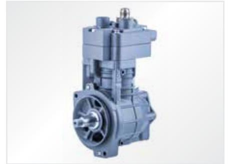
The **aluminum compressor casing** reduces the weight by up to 35% compared with the previous model. The water cooling system incorporated in the cylinder also cuts the temperature by up to 50 °C. This reduces oil contamination, improves air quality and prolongs the operating life of the air drier cartridge.
