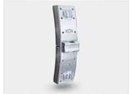
The **LL composite brake block** significantly lowers the rail noise of freight cars compared to conventional cast iron brake blocks. The same goes for the K pad, which is used for new freight cars. 10 years after the introduction of the first K pad, the second generation has now been launched, offering improved wheel wear.
