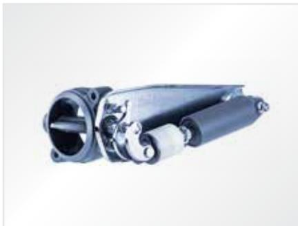
The **engine retarder** ensures the vehicle maintains a constant speed on downhill gradients independently of the engine load and speed. It controls the exhaust mass flow and plays an important role in reducing wear and tear on the service brake.
