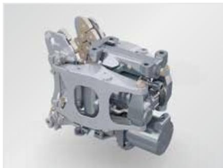
The **compact brake caliper** prevents disruptive noise and saves up to 120 kg per bogie, thus lowering the entire vehicle's noise levels and energy consumption.
