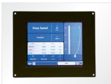
The **iCOM Assist (LEADER) driver assistance system** supports drivers, enabling them to operate trains as energy-efficiently as possible, minimizing wear, and still arriving safely and punctually. iCOM Assist typically makes it possible to save 10% of energy costs.
