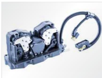
The **shifting module for the dual clutch transmission** of a heavy-duty truck ensures rapid shifting without any interruption in the flow of power, which means added comfort for the driver and fuel savings for the fleet operator.
