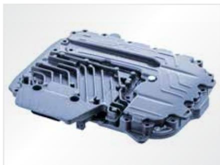
The **mechatronic transmission control system** reduces fuel consumption by ensuring that the engine is always running in the optimum operating range. The unit consists of an electronic control module, a pneumatic module and a sensor unit that registers the gear selected as well as the temperature and speed of the transmission.
