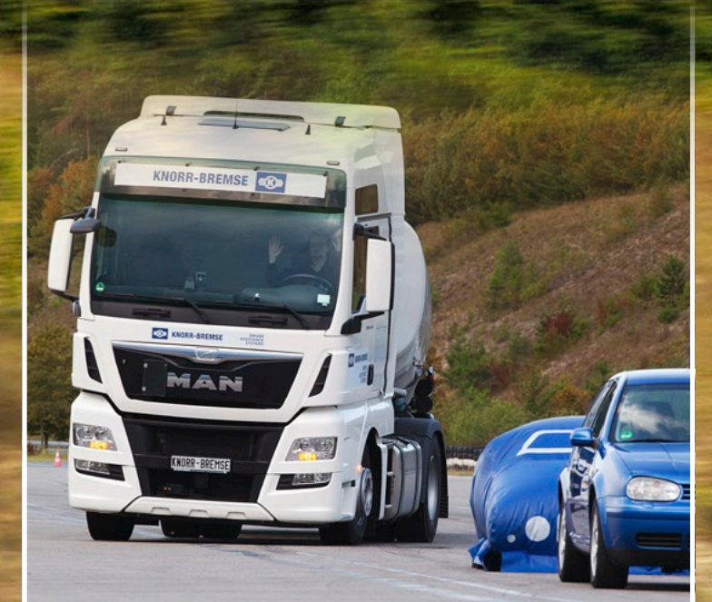
The Automatic Emergency Braking System (AEBS) prevents rear-end collisions in tailbacks without driver intervention.
