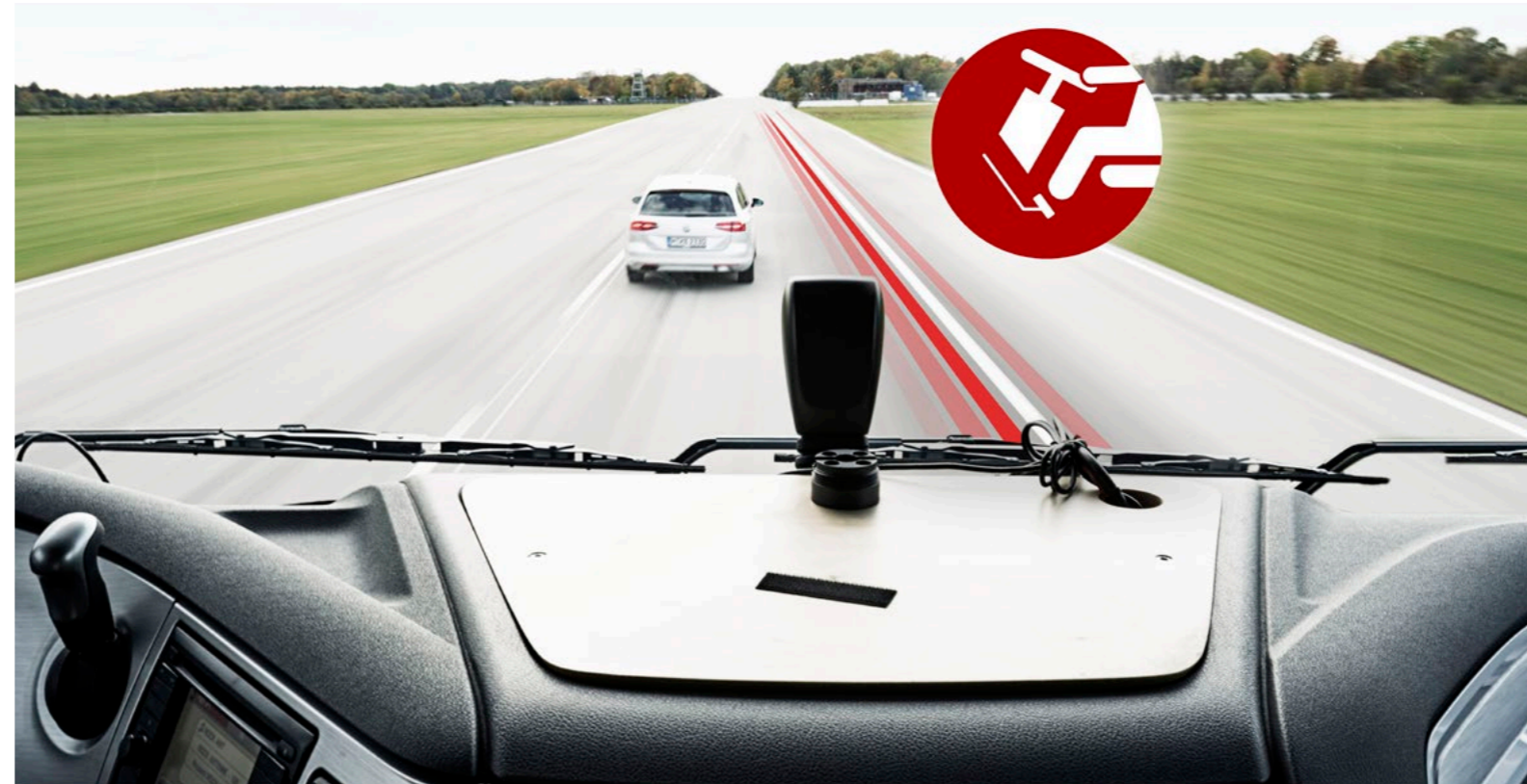
The Highway Departure Braking function brakes the vehicle on the shoulder if LDW is ignored.
