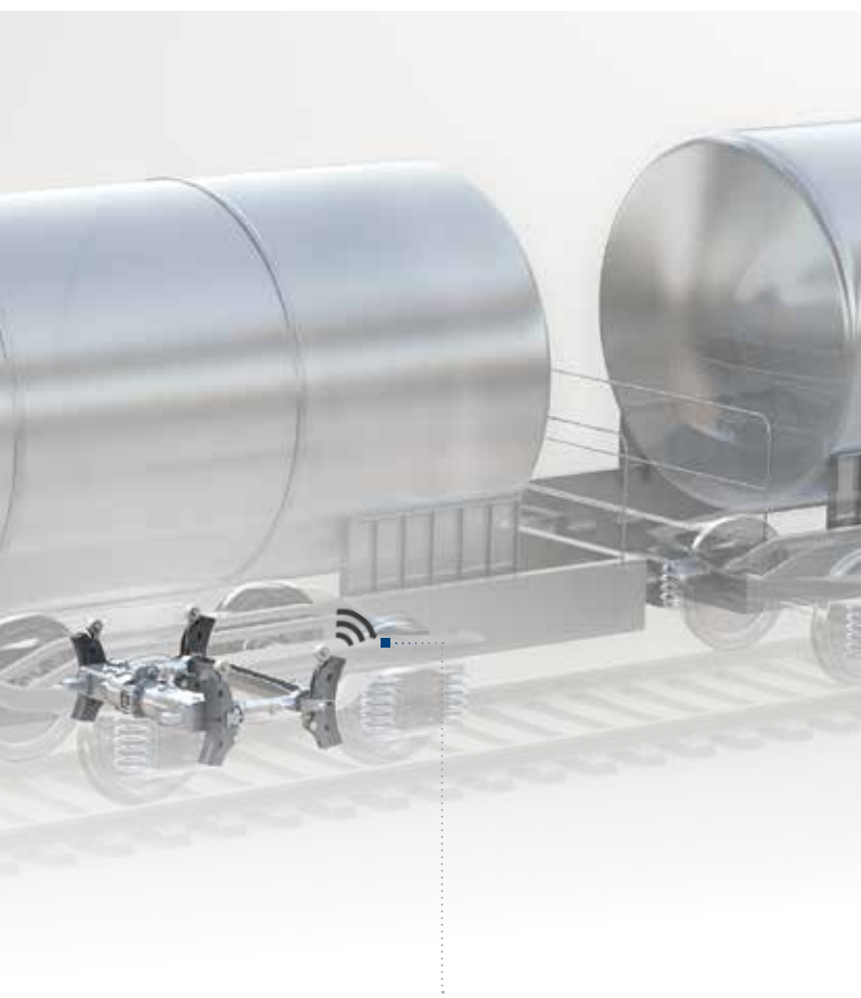
Sensors on bogie and car body for wagon and track monitoring
