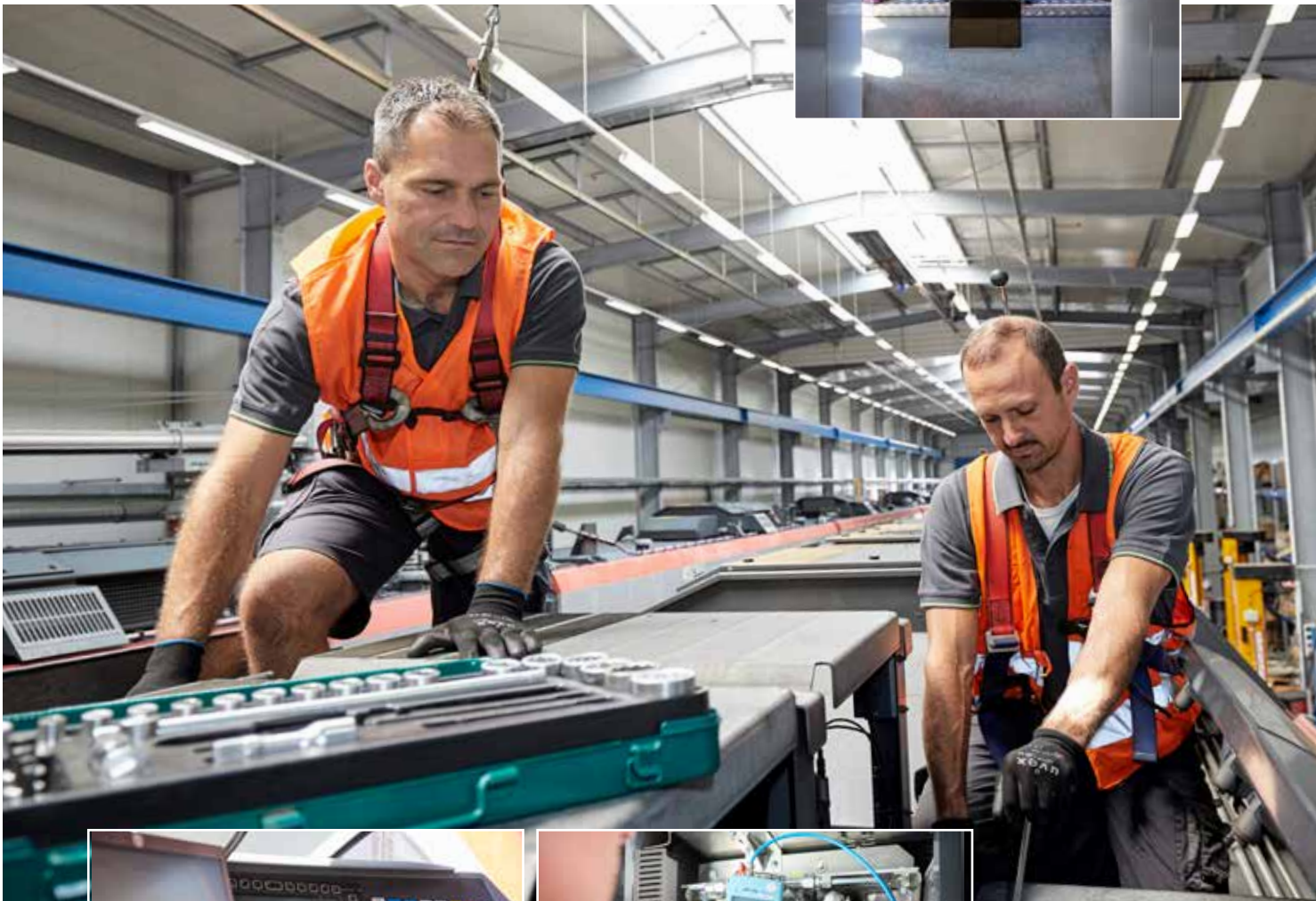
Thomas Thiele (l) and Michael Obermaier on the roof of a FLIRT preparing the complete compressor housing for replacement ▼
