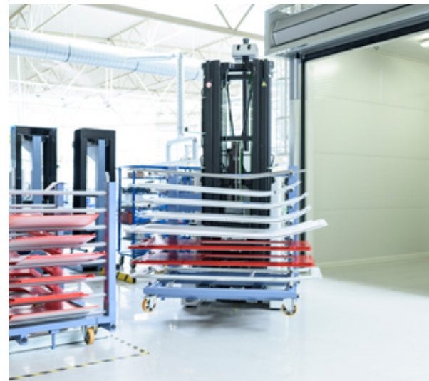
Fully-automated transportation of door leaves largely avoids the risk of damage (right).
