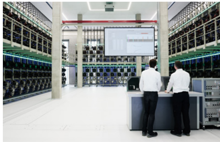
The Universal Train Test Rig can simulate the braking of entire passenger and freight trains.
