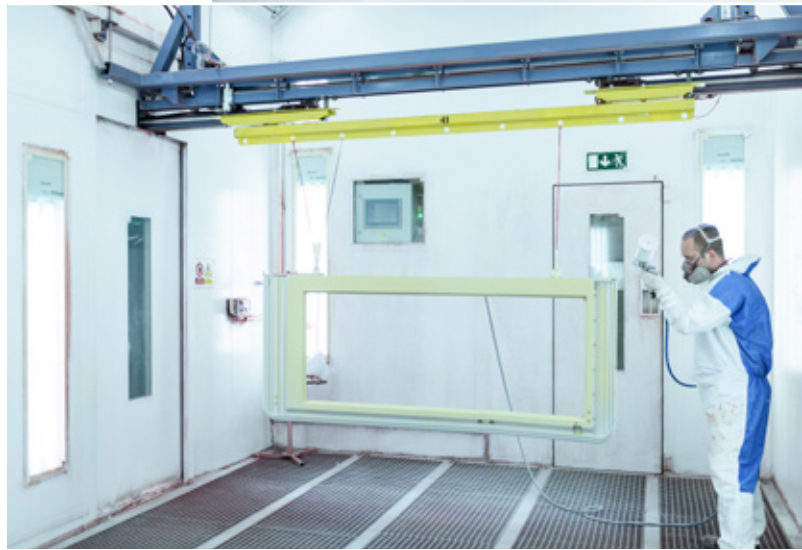
The paint chambers have state-of-the-art equipment for efficient manual painting.
