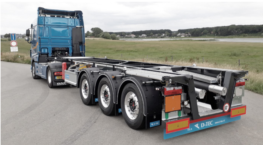
D-Tec's new flagship CC 2030 trailer – featuring Knorr-Bremse braking technology – will be on display at the IAA.
