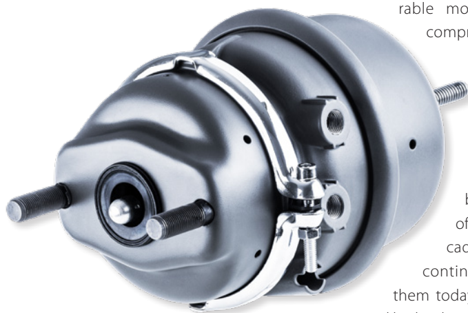
One for all: the NG4+ diaphragm brake cylinder (similar to pictured unit).
