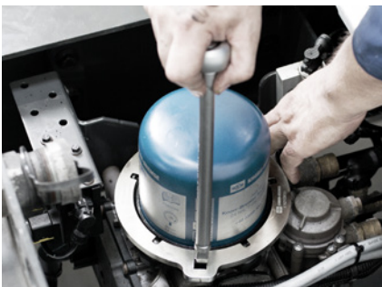
Special tool with bayonet ring for the maintenance of air dryer cartridges, in operation.
