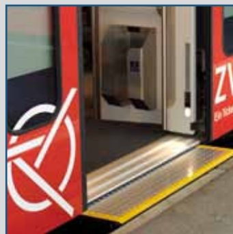
Sliding steps and gap bridges
