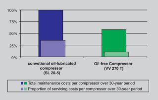
Total maintenance costs per compressor over 30-year period Proportion of servicing costs per compressor over 30-year period The oil-free compressor offers considerable reductions in servicing and maintenance costs. In the example above, based on average costs for 1,500 operating hours per year, overall maintenance costs are cut by almost 40% and servicing costs by almost 70%.
