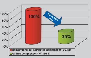
Various noise reduction measures, combined with extremely low-vibration operation, make the oil-free version significantly quieter than conventional
