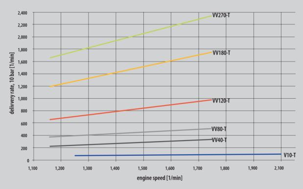
Depending on the engine speed the oil-free compressors deliver up to 2,350 l/min at 10 bar.
