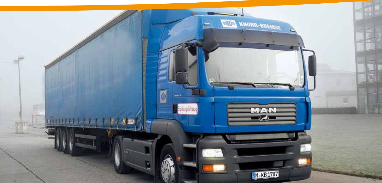
The test vehicle: a 430 hp MAN TGA semitrailer rig with automated transmission.
