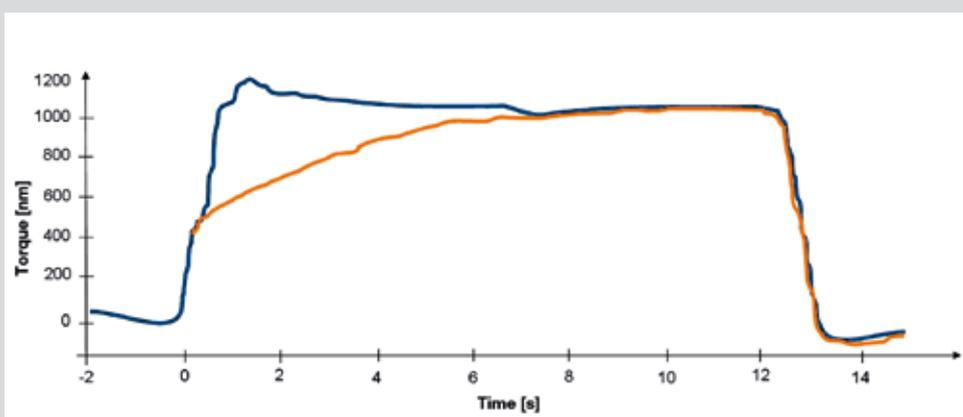
With PBS (blue), a turbodiesel engine develops boost pressure and torque much faster than without (orange).
