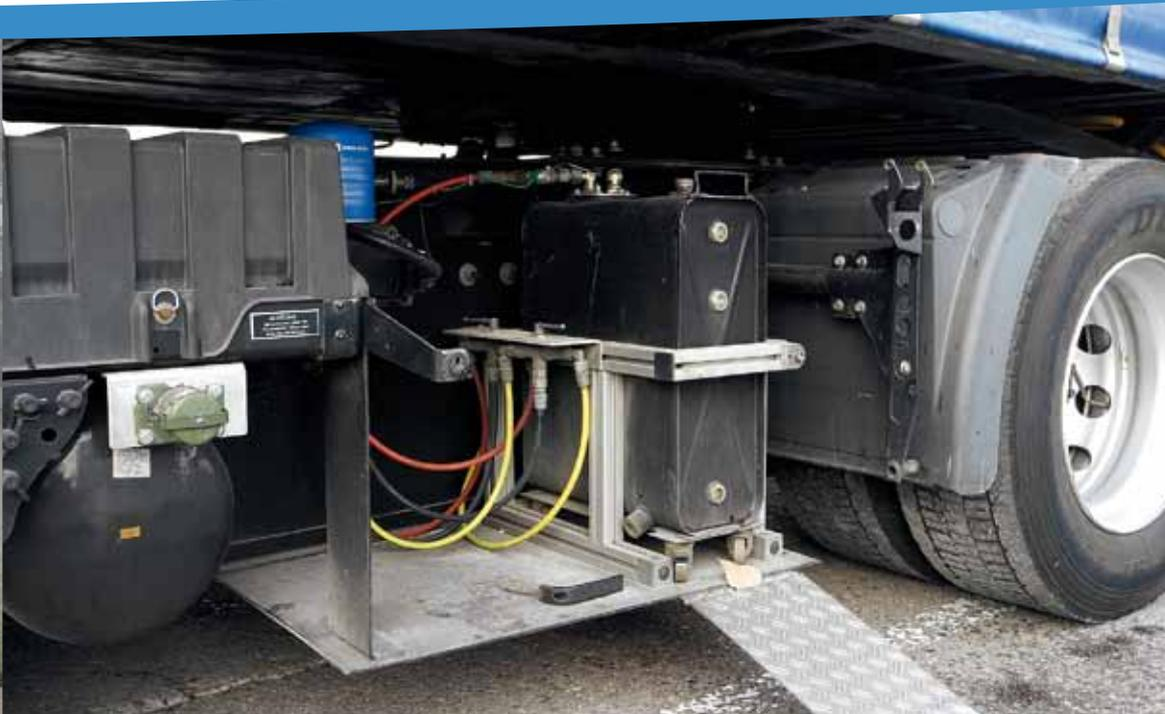
2 Precise fuel consumption measurement: the 30-litre test tank was weighed before and after each lap, then refilled.
