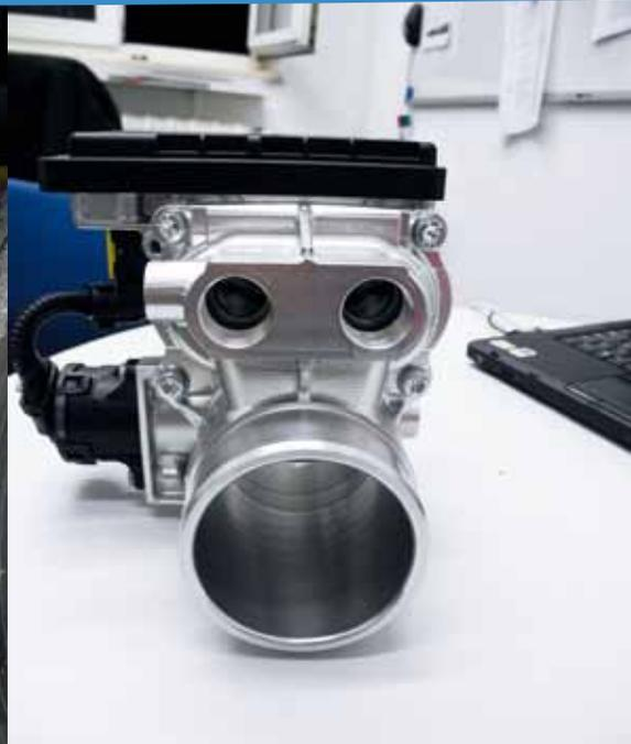
The PBS system is based on a pipe, a throttle valve, two temperature sensors, two diaphragm valves, a processor – and lots of development work.
