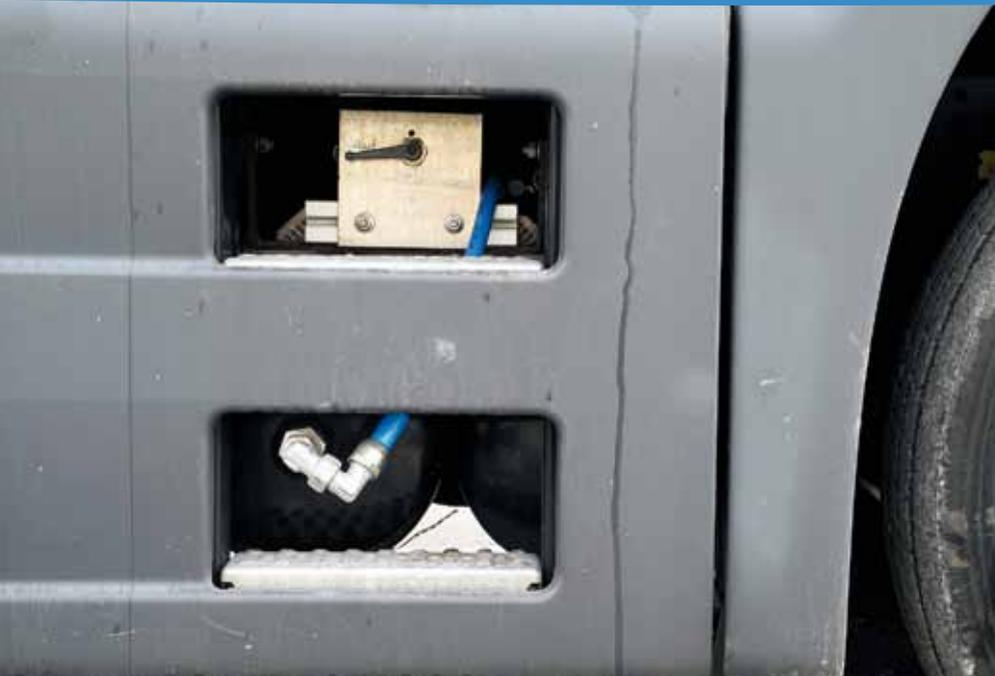
Two supplementary air tanks, providing 80 litres of additional compressed air capacity, were fitted behind the side panels.
