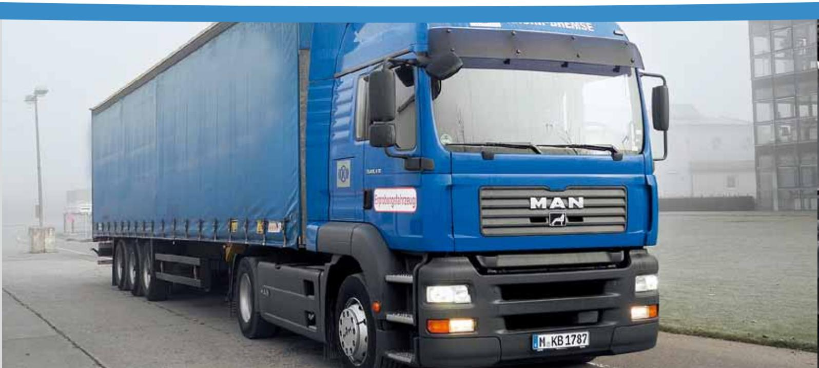
1 The test vehicle: a 430 hp MAN TGA semitrailer rig with automated transmission.
